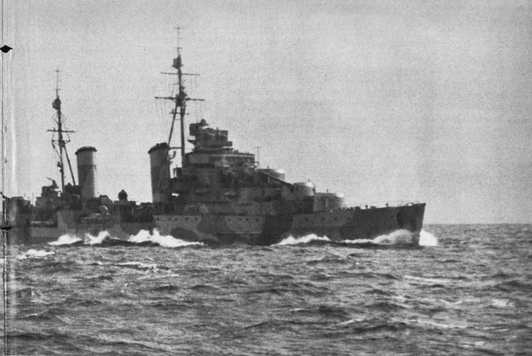
THREE TURRETS FORWARD, TWO AFT. CHARYBDIS GROUP OF DIDOS CARRIES EIGHT IN TWIN MOUNTS. BOTH HAVE WIDELY SPACED RAKING STACKS
